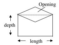
Not over 100 mm in depth - opening not over 140 mm in length
